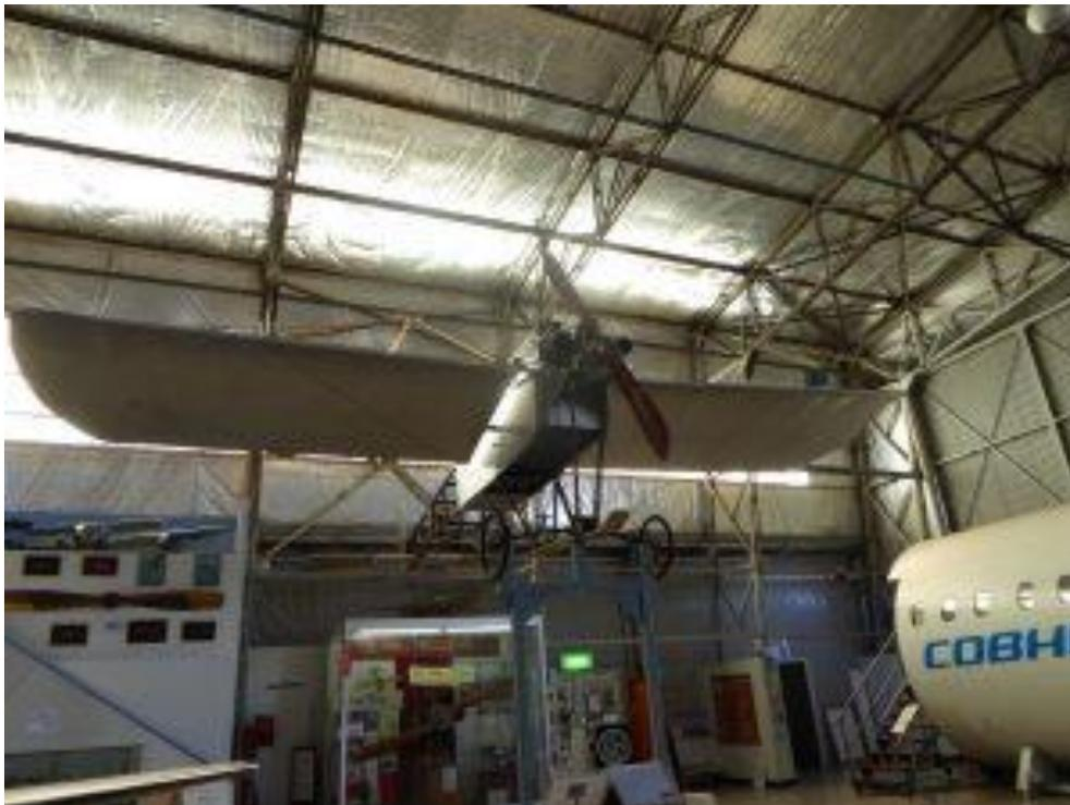
The Cessna replica is fitted with a replica three cylinder Anzani engine, which also powered the Bleriot. The wooden propeller was made from scratch by one of our volunteers, Jim Piscioneri.
